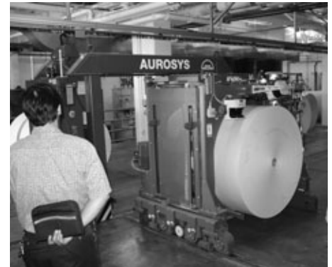
Robot travels on track carrying roll of paper to one of the presses.
