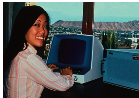
This user is operating the ALOHAnet hub machine, which uses a random access protocol to transmit packets over a shared channel.
